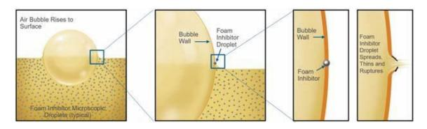
Performance Plus<sup>®</sup> EP Gear Oil (MD) contains a specialty blend of additives that enhance surface tension and maintain film strength which provides excellent resistance to foaming. The strength of the additive package will break down foaming air bubbles a quickly as they form.
