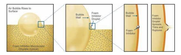
Performance Plus<sup>®</sup> EP Gear Oils (EHV) contain a specialty blend of additives that enhance surface tension and maintain film strength which provides excellent resistance to foaming. The strength of the additive package will break down foaming air bubbles a quickly as they form.
